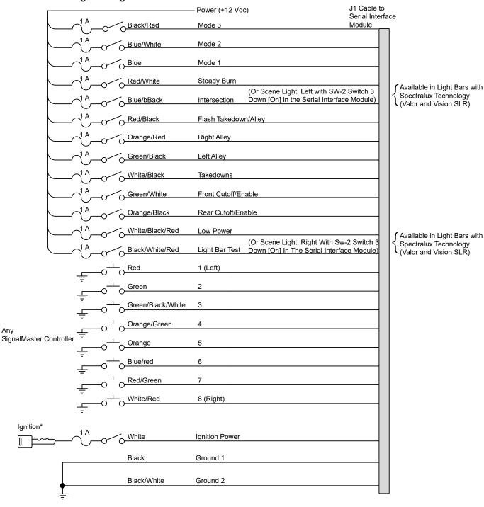
Figure 5 SignalMaster control functions wired to 12 Vdc for External Control
