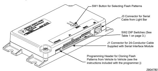
Figure 1 Connectors and switches on the Serial Interface Module
