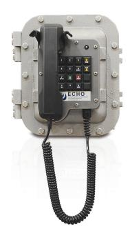
Federal Signal Model E1 Series ECHO Intercom Stations, UL, cUL and CE listed, provide safe and efficient two-way voice communications in ECHO Digital Intercom Systems. The E1 Series ECHO Station is designed and approved for use in Hazardous Areas including Class I, Division 1, Groups C and D; Class II, Division 1, Groups E, F and G; and Class III.
