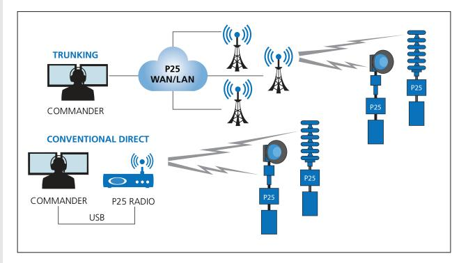
Control Point computers hosting the Commander software can now connect to a P25 trunked land mobile radio interface via an Ethernet connection. Control points utilize a broadcast functionality to quickly and efficiently communicate with all remote controllers for All Call and Group activations. IP unicast to individual remote sites is used for individual activation and polling requests to minimize radio traffic in a multi-site system.
