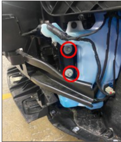
Figure 6 Driver Side Frame Bolts
