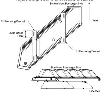
Figure 2 Light bar with brackets installed
