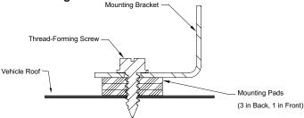
7. Ensure that all fasteners are tightened properly.
