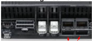
Figure 1 Convergence Network Ports
