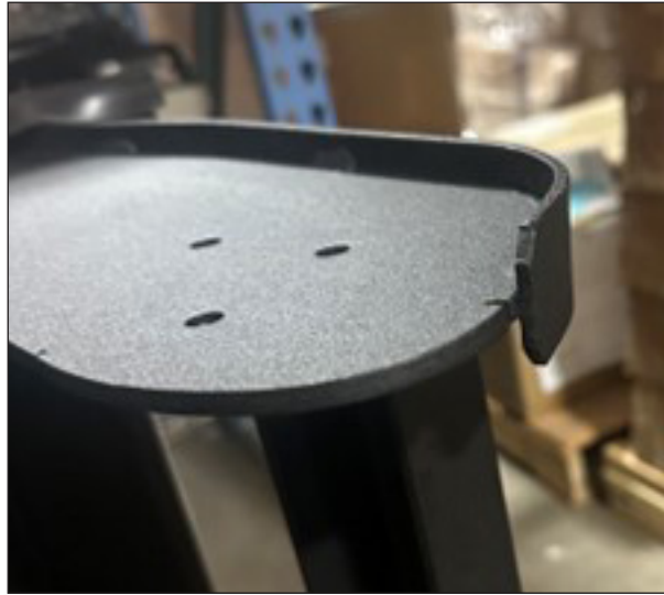
Figure 2 Slide molding onto metal upright
