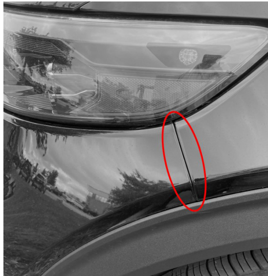
Figure 6 Fascia fender fasteners to be removed
