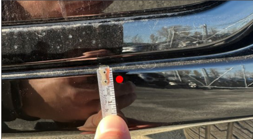
Figure 6 Front post vertical measurement
