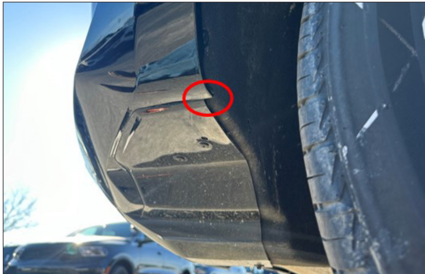
Figure 7 Fascia feature/ measurement starting point
