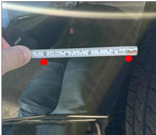
Figure 9 Side post horizontal measurement
