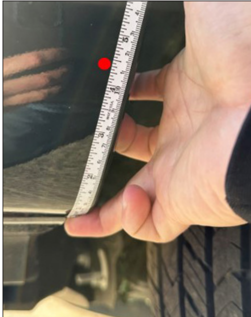
Figure 8 Side post vertical measurement
