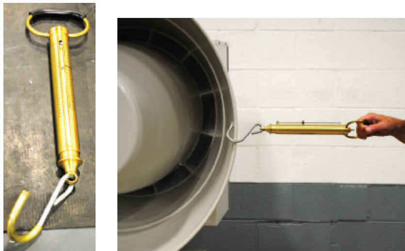
Figure 16 Spring scale attachment to siren
