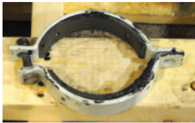
Figure 7 Clutch band assembly
