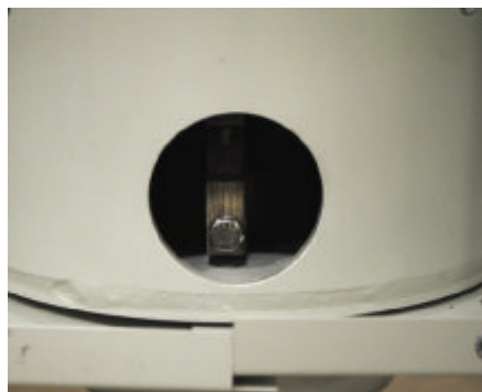
Figure 5 Collector ring access hole
