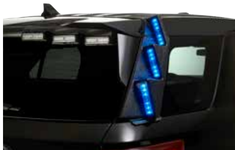
D-Pillar lighting system ELSD-FPIU20RBA installed on a 2020-2024 Ford Police Interceptor Utility.
