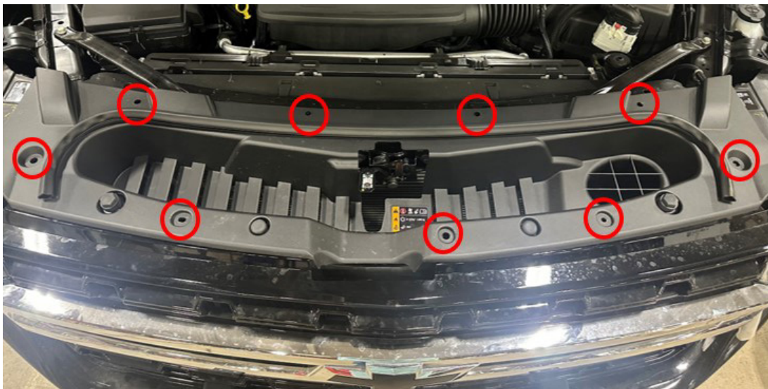
Figure 9 Intake air splash shield fasteners to be removed
