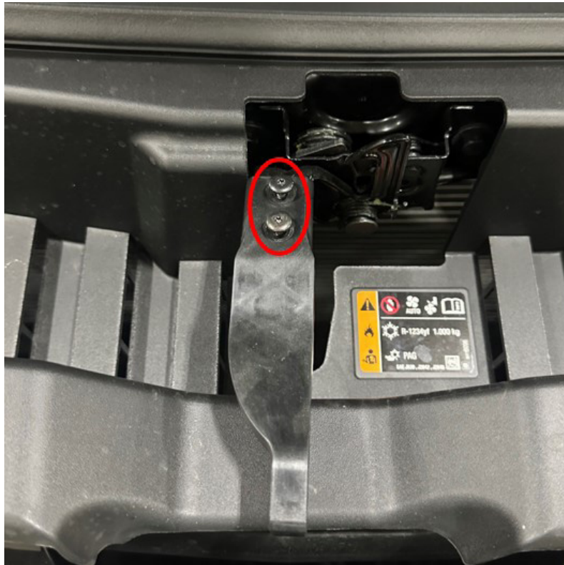
Figure 9 Intake air splash shield fasteners to be removed
