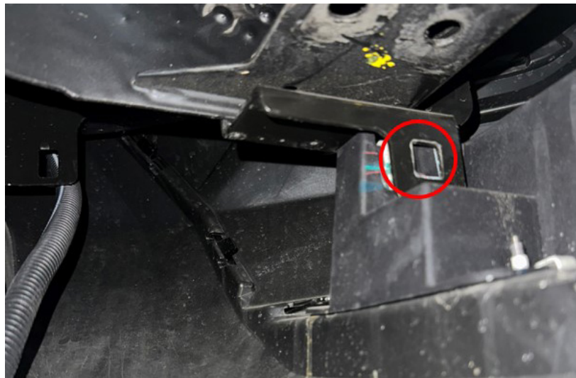
Figure 7 Fascia fasteners to be removed from fascia support brace behind wheel well
