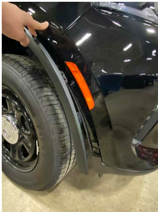
Figure 4 Remove the fascia retaining fender clips and partially remove the fender trim from the front fascia
