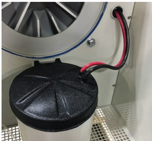
Figure 20 Wire ties around four gauge wires
